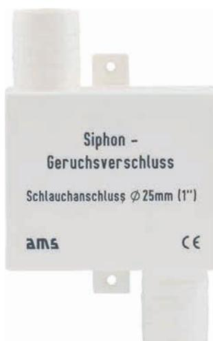
The siphon odour trap prevents smells from the waste water tank. It is simply inserted into the severed wastewater hose. It is cleaned by rinsing out with water. The siphon odour trap is available for hose sizes of Ø 19 mm (3/4") and of Ø 25 mm (1").
