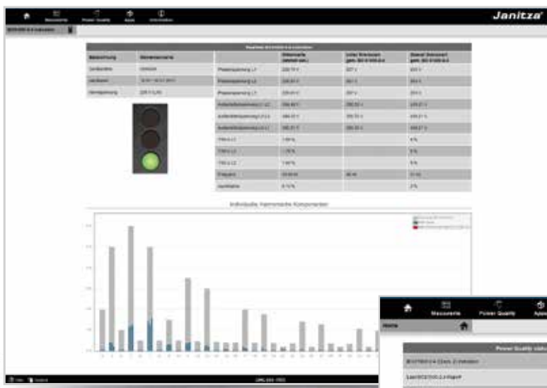
Fig.: IEC 61000-2-4 analysis with traffic-light principle
