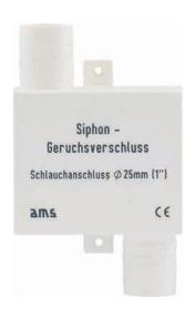
The siphon odour trap prevents smells from the waste water tank. It is simply inserted into the severed wastewater hose. It is cleaned by rinsing out with water. The siphon odour trap is available for hose sizes of  $\varnothing$  19 mm (3/4") and of  $\varnothing$  25 mm (1").
