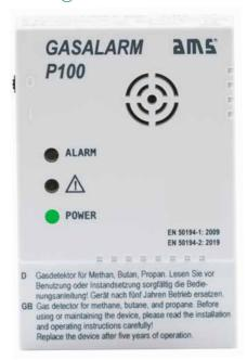
The GASALARM P100 detects liquefied petroleum gas (propane/butane) and town gas/natural gas (methane) well before an explosive mixture occurs and warns with an optical and acoustic alarm.
