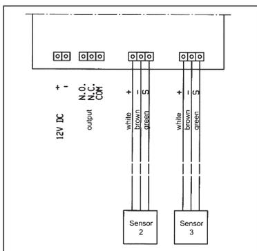
**Attention must be paid to connecting the wires to the correct terminals.**
