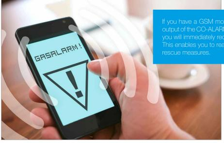
If you have a GSM module, you can connect it to the relay output of the CO-ALARM S/200-C. If a gas alarm is triggered, you will immediately receive an SMS on your mobile phone. This enables you to react promptly and initiate all necessary rescue measures.
