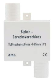
The siphon odour trap prevents smells from the waste water tank. It is simply inserted into the severed wastewater hose. It is cleaned by rinsing out with water. The siphon odour trap is available for hose sizes of  $\emptyset$  19 mm (3/4") and of  $\emptyset$  25 mm (1").
